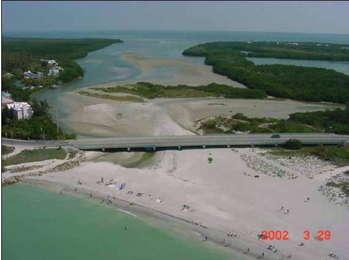
Figure 23. Blind Pass, a wave-dominated inlet, shown after having closed naturally. Due to small tidal prisms, wave-dominated inlets tend to periodically close. When open, these types of inlets contain smaller ebb-tidal shoals and are a less suitable sand source than their larger counterparts (tide-dominated and mixed-energy inlets). (Photo provided by the Lee County Government – Robert Neal).
