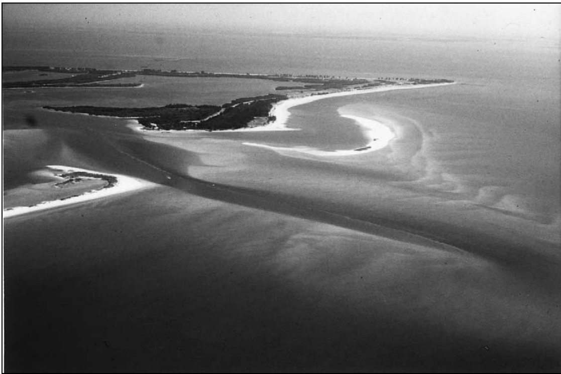
Figure 22. Bunces Pass, one of the inlets that connect Tampa Bay to the Gulf of Mexico, is an example of a tide-dominated inlet with a well developed ebb tidal shoal. (From Davis et al. , 2003).
